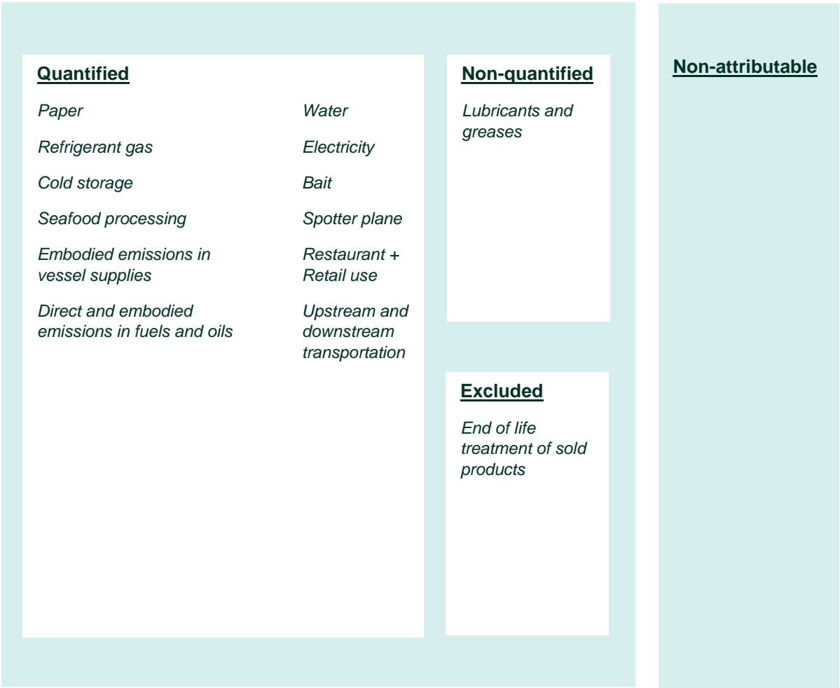
Figure 3. Austral Fisheries’ emission sources which have been used in the Life Cycle Assessment of seafood products. Note that all emissions sources lie within the existing organisation inventory.
