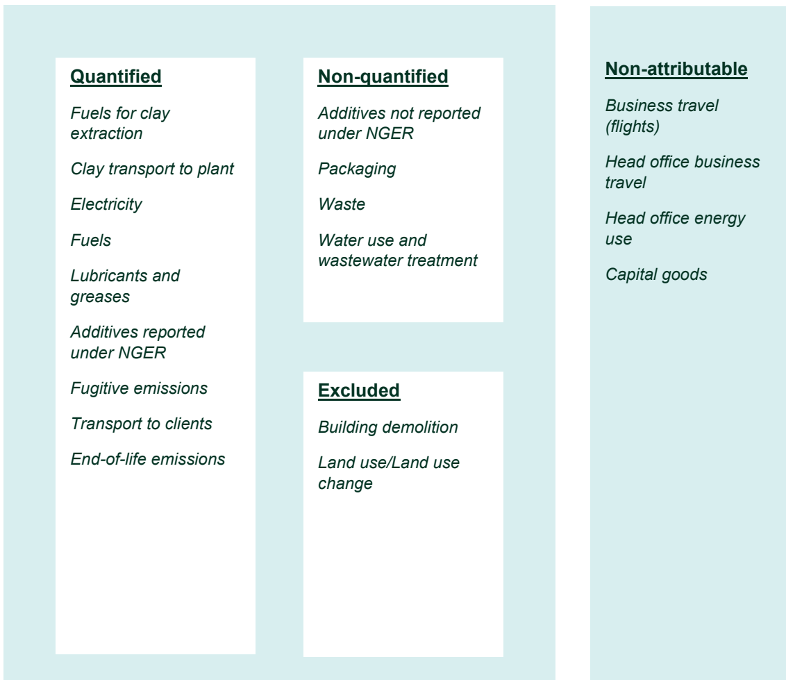
Figure 3. Attributable and non-attributable emission sources included and excluded in the LCA.
